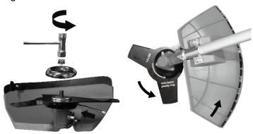
To remove the blade, insert a metal locking tool through the hole on the side of the drive sprocket and on the drive shaft. Loosen the clamp nut, then remove all parts.
