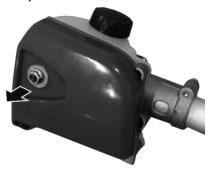
Install the guide bar on the tool and pass the chain over the wheel. Install the cover and tighten the fixing screw.
